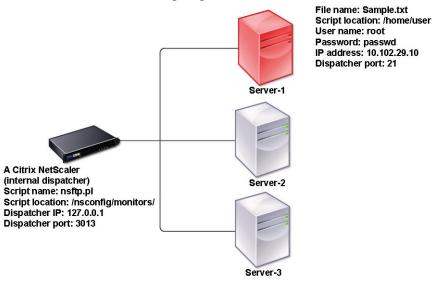
Using a user monitor with the internal dispatcher
