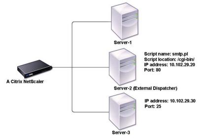
Using a user monitor with an external dispatcher
