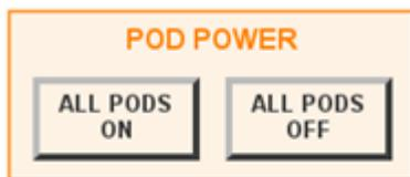
This controls the power to the displays at the pods. Pushing the ALL PODS ON button will turn on all of the displays and automatically enables SEND TO PODS ON (see below).
