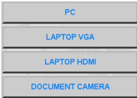
This controls the source that is being projected, shown on the SMART Podium's screen, and sent to pods. PC uses the provided computer. LAPTOP VGA and LAPTOP HDMI are if you connected a personal computer via either the VGA or HDMI cables. The DOCUMENT CAMERA button will display the image from the document camera. A document camera can be checked out from the front desk.
