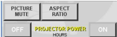
The PICTURE MUTE button functions similarly to the SEND TO PODS OFF button. The ASPECT RATIO button changes the display size. Auto is recommended. The ON and OFF buttons turn on or off the projector power. There is a 90 second cool-down after turning the projector off
