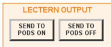
When SEND TO PODS OFF is selected, the image on the projector will not be able to be seen on the pods. When it is ON, the pods can view the image (even if the projector is off)
