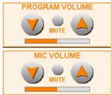
These buttons control the volume. The MIC VOLUME buttons control the volume for the microphone. The PROGRAM VOLUME buttons control the volume coming from the computer.
